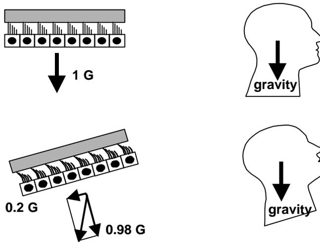
Equivalence between gravity and linear accelerations
