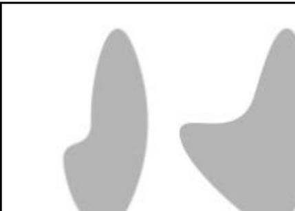
The diagram shows two beam patterns. The left one is a standard beam. The right one is a beam that is curved to follow the direction of the road.
