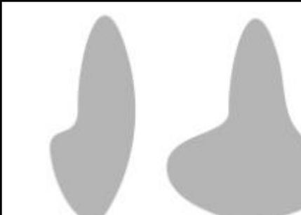
The diagram shows two beam patterns. The left one is a standard beam. The right one is a beam with a wider, lower spread at the bottom.
