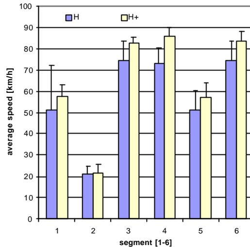
**Figure 5. Speed control: the influence of the height of the driver viewpoint.** The average speed along the different segments of the circuit for two configurations of the simulation environment: H standard height of the driver viewpoint, H+ increased height of the driver viewpoint.
