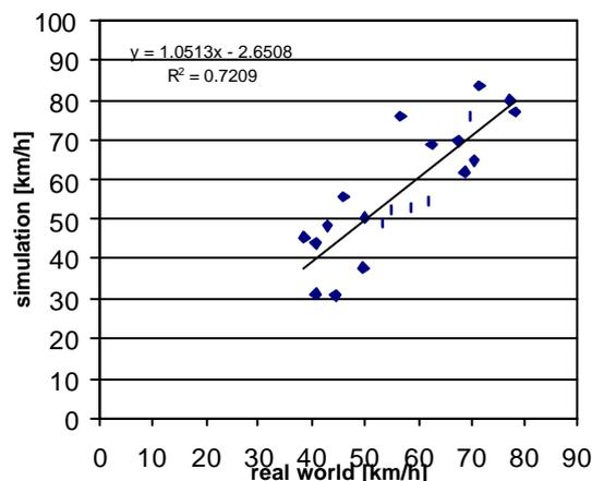
**Figure 3. Speed control: relationship between simulator and real-road speeds.**
