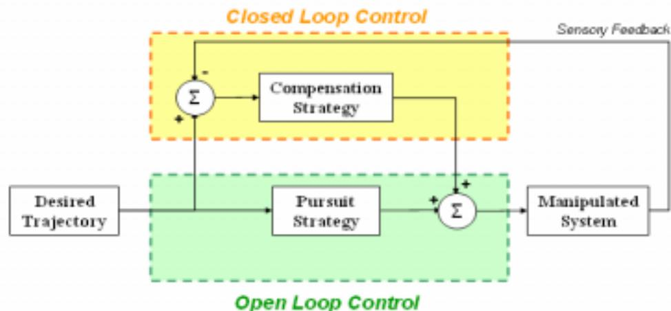
**Figure 5:** General tracking model architecture
