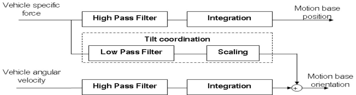
Figure 3 - Classical Motion Cueing Algorithm Filter Structure
