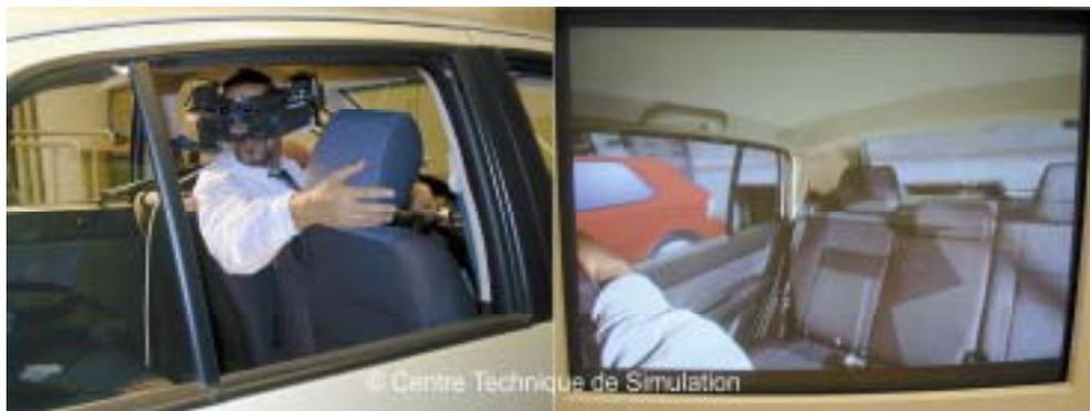
Figure 3. Renault's Augmented Reality (AR) simulator used for vehicle architecture studies
