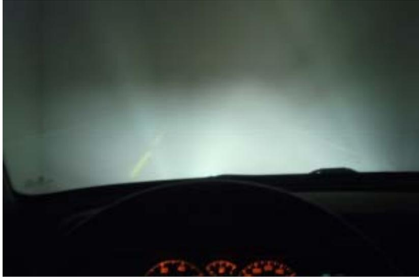
Figure 2. Headlight simulation in foggy conditions with Renault's headlight simulator
