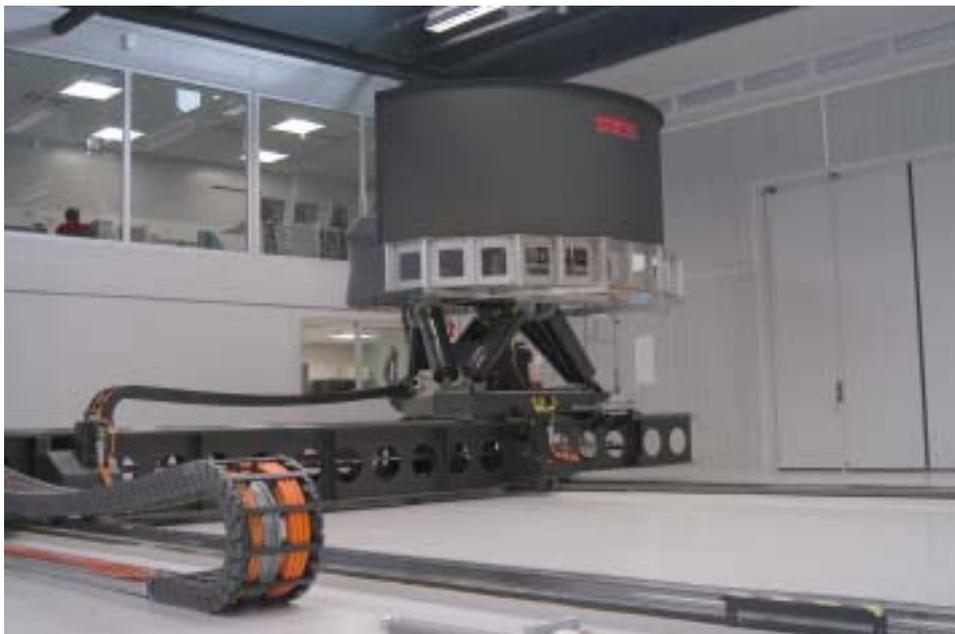
Figure 1: Renault's high performance ULTIMATE simulator
